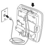
6. Align the mounting slots on the base with the mounting screws on the wall. Push in and down until the phone is firmly seated.
